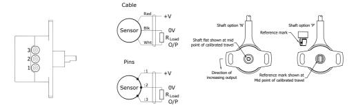
**Mechanical Mounting:** Flange mounted. The sensor should be mounted with minimal axial and radial loading on the shaft for optimum life. It is recommended that the Ø 4 mm shaft option is coupled to the drive using a flexible coupling - see drawing P501-11.
